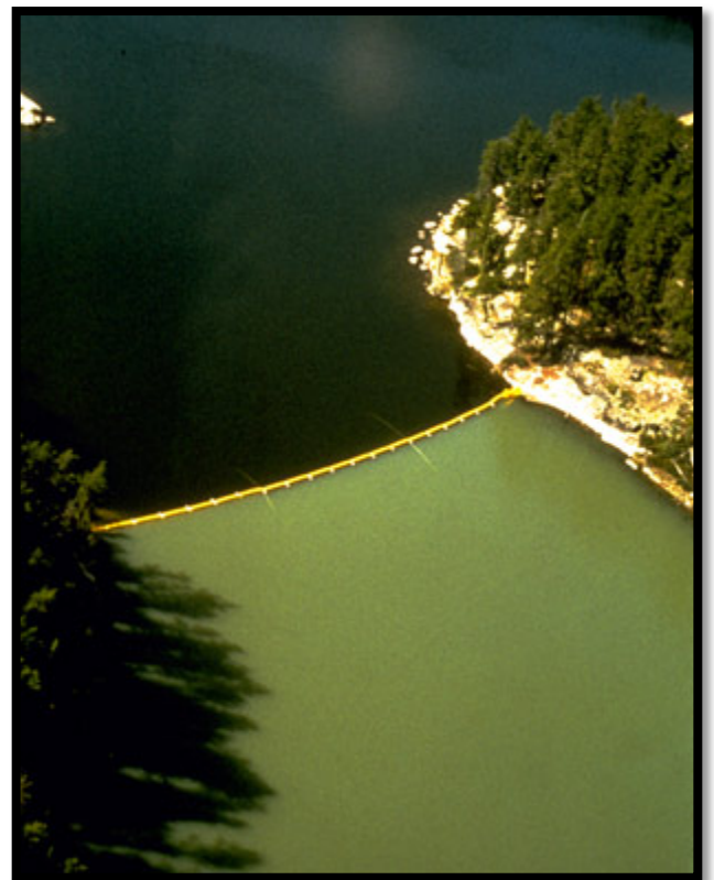
Figure S.2.5. Phosphorus-enriched versus unenriched water. Note: Enriched water (below the curtain) is highly turbid. Canadian Experimental Lake Area. Source: http://saveela.org .
